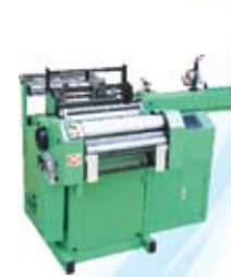
Introducing JYP 500 suitable for making 500mm width fabric (rigid) Elastic) with electronic take up.
